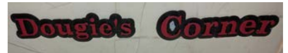
ANOTHER CINEMA 4D GENERATED MODEL AND THEN 3D PRINTED. CINEMA 4D TREATS TEXT AS SPECIAL OBJECTS THAT CAN BE EXTRUDED AND RESHAPED VERY EASILY
